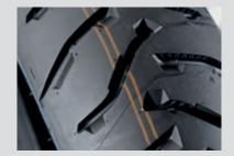
UTILITY OF THE SERRATIONS ON THE GROOVE SIDES In the course of the tyre's working life, the way these 3D serrations wear enables the amount of rubber in contact with the ground to remain beneficial to grip in dry weather, while the additional edges contribute to grip on wet roads.
