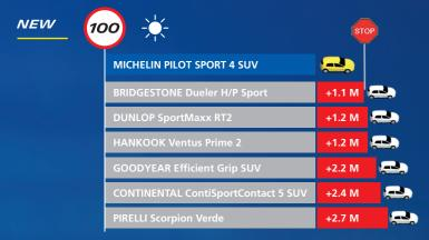
(1) Dry braking test, between 100 and 0 kph: conducted by TÜV-SÜD Product Service, on Michelin's request, in September 2018, on dimension 235/60 R 18 107W on Audi Q5 2.0 TDI.
